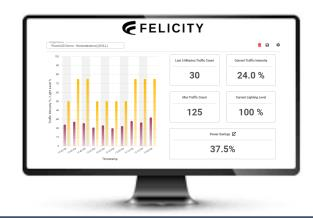
The relative traffic intensity is constantly monitored live in Felicity Connect. When predefined traffic intensity thresholds are crossed, a predefined corresponding dimming level command is generated and sent to the Smart Lighting platform for the assigned group of streetlights.
